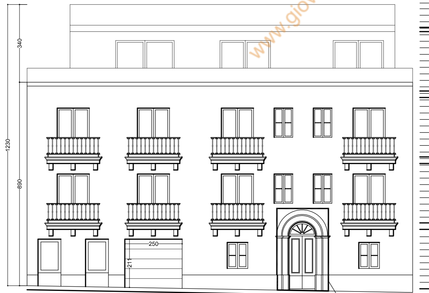
Front Elevation 1:100 As Proposed Unpainted Franka Stone Facade White PVC Apertures and Railings
