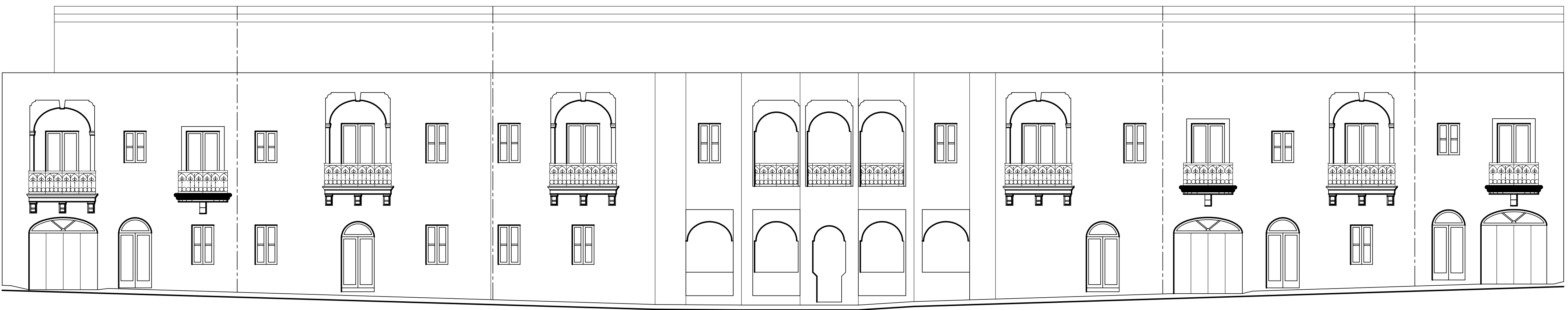
○ Front Elevation 1:100 As proposed (clean copy) Unpainted Franka Stone Facade PVC Apertures timber texture color as per G52 of DC15 Wrought Iron railing painted as per G52 of DC15
