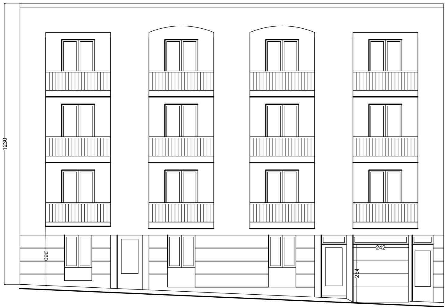
Front Elevation Scale 1/100 Unpainted Franka Stone Facade White Aluminum Apertures and Railings
