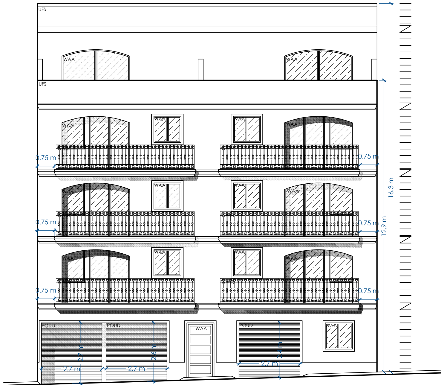
FRONT ELEVATION PROPOSED Scale 1:100
